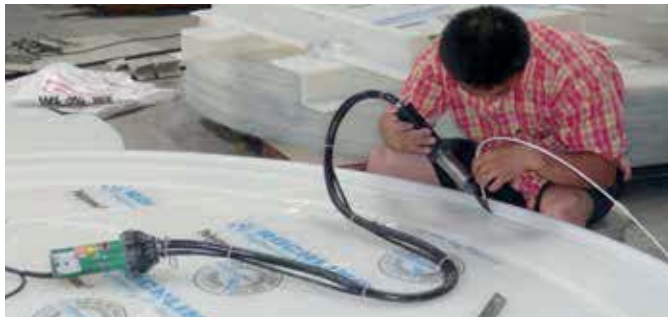
The MINOR blower as an air supply for the DIODE PID.
