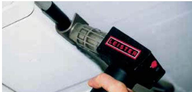
Shrinking cable connections with the GHIBLI.
