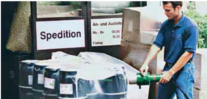
Flameless shrink-wrapping of pallets and bulk goods with the FORTE S3.
